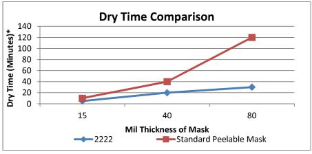
\*Dry time is the time until the mask could be easily removed, in one piece, from the substrate. Beads of mask were approximately 4 inches in length.
